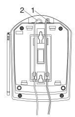
Place the Base Unit on the two screws in the wall and slide downward to secure.
