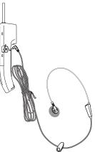
Note: The earpiece and microphone in your cordless handset are disabled when the headset is plugged in. We suggest you use the Uniden HS900 Headset. This headset is specifically designed to deliver optimum performance. Use of other headsets may result in less than satisfactory performance.
