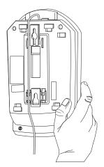
Plug the short telephone cord into the phone and the GTE Wall Plate jack. Place the Base Unit on the two posts of the wall plate and slide downward to secure.
