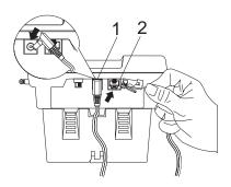
Thread the AC Power Cord through the clip on the base stand, and place the Base Unit on the desk or table top.
