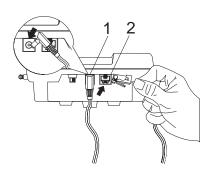
Place the power cord in the left molded channel on the bottom of the Base Unit.
