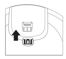
2. Flip the Retainer over so the tab is facing up, and slide the Retainer back into the Base Unit.
