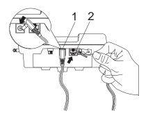
Place the power cord (1) in the right molded channel and the telephone cord (2) in the left molded channel on the bottom of the Base Unit.
